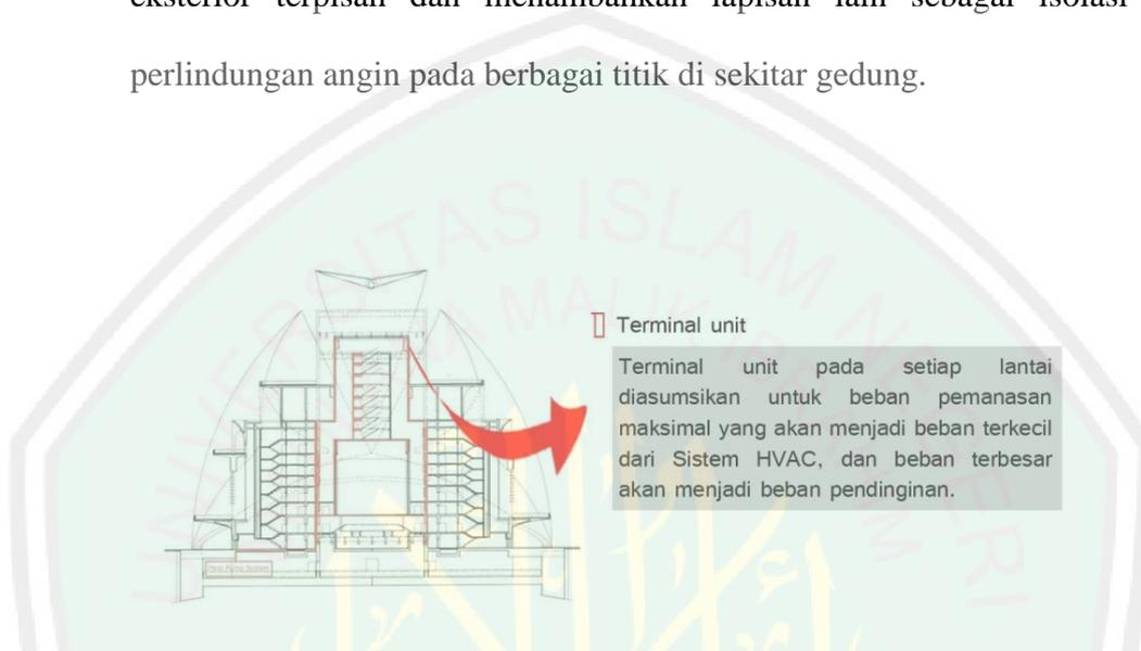
Gambar 2. 42 Perletakan Terminal Unit Sistem HVAC (Sintesa Teori, 2016)
