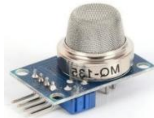
Gambar 2.9 Sensor gas (MQ-135) (Pratama & Nurpulaela, 2024)
