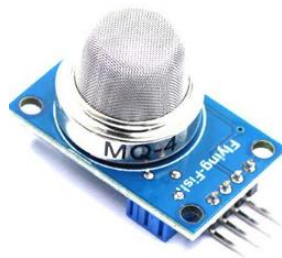
Gambar 2.6 Sensor gas (MQ-4) (Diantoro & Rahmadewi, 2020)
