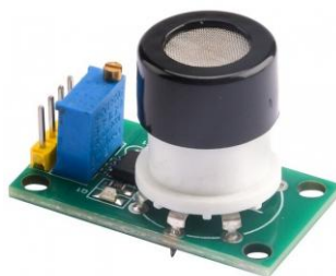
Gambar 2.11 Sensor gas (TGS-813) ( https://pousadamariola.com.br )
