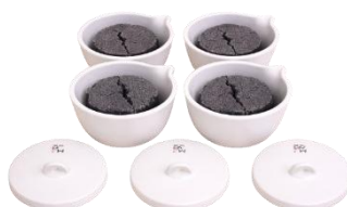
Calcined at 500°C for 3 hours
