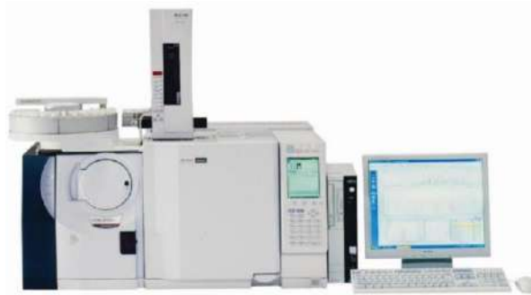
Gambar 2.1 Alat Gass Chromatography-Mass Spectrometry (GC-MS)
