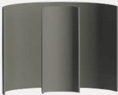
MID STRUCTURE - Ring Beam & Radial Beam
