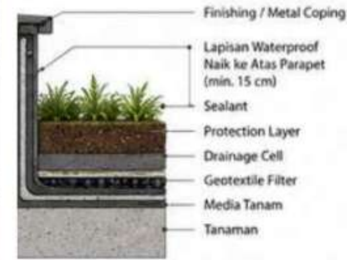
DETAIL DRAINASE ROOF GARDEN
