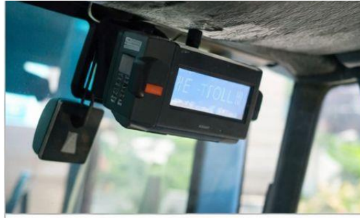
Figure 4.2 Installation of On Board Unit (OBU)
