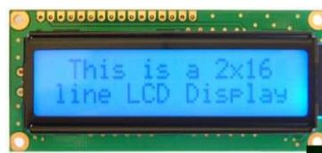
Gambar 2.9 LCD 16x2 pin
