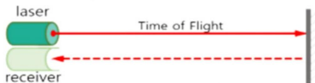
Gambar 2. 8 Cara kerja LiDAR ToF (Sumber: Fikri & Rivai, 2019)
