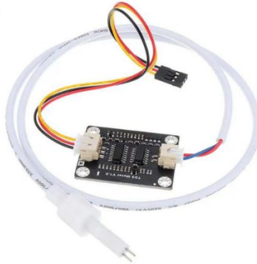
Gambar 2. 5 Sensor TDS ( Total Dissolved Solids )
