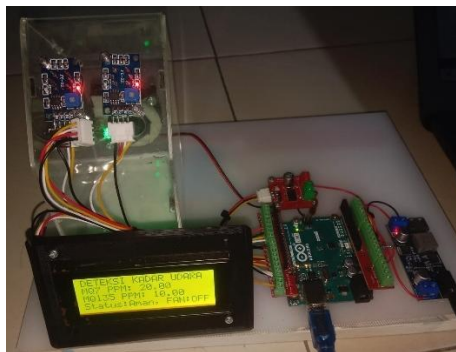
Gambar 4. 1 Rangkaian Alat Monitoring Kadar Gas CO dan CO 2
