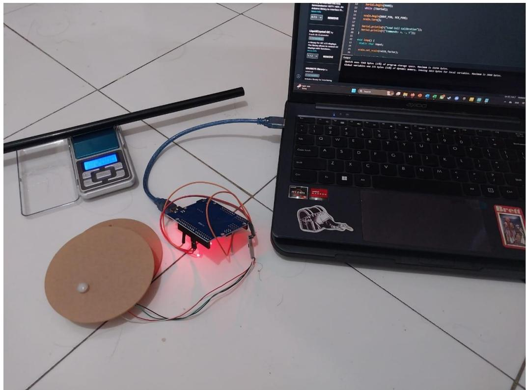
Gambar 4. 2 Proses Kalibrasi Sensor Load Cell
