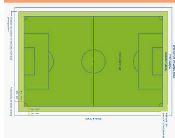
Gambar 2.12 Ukuran Lapangan Sepak Bola+ Area Bantu Sumber : FIFA football stadium technical recommendations and requirements [15]
