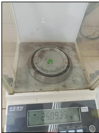
Penimbangan garam logam \text{NiCl}_2 \cdot 6\text{H}_2\text{O}
