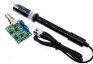
**Gambar 2.4** Sensor pH PH4502C
