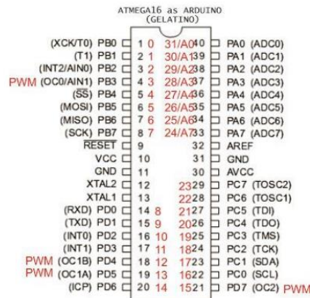
Gambar 2.5 Pin Map Arduino (akuarduino.blogspot.com)
