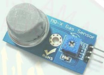
**Gambar 3.18.** Sensor Gas MQ2
