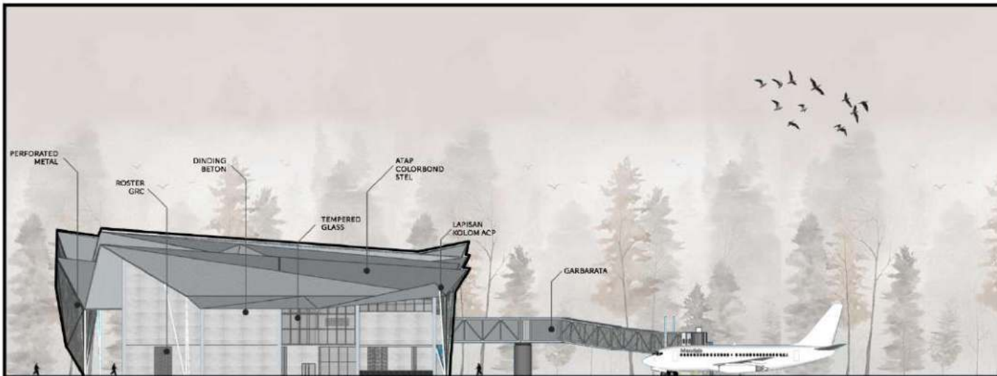
TAMPAK KANAN TERMINAL SKALA 1:500
