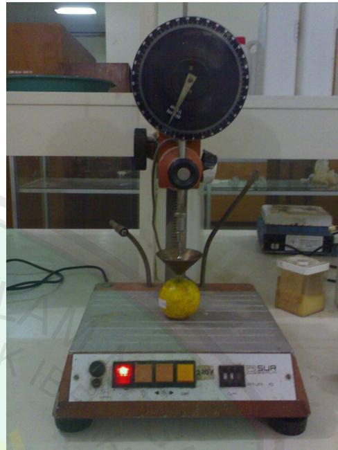
**Gambar 2. Penetrometer**
