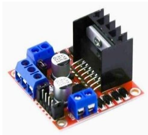
Gambar 2.5 Modul Driver Motor L298N
