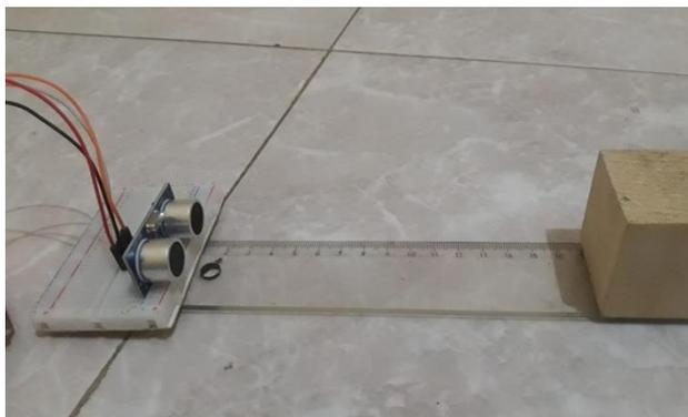
**Gambar 3.4** Kalibrasi Sensor Ultrasonik HYSRF-05
