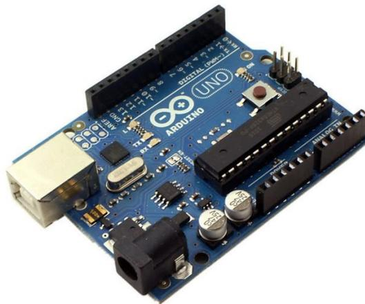
Gambar 2. 4 Board Arduino Uno
