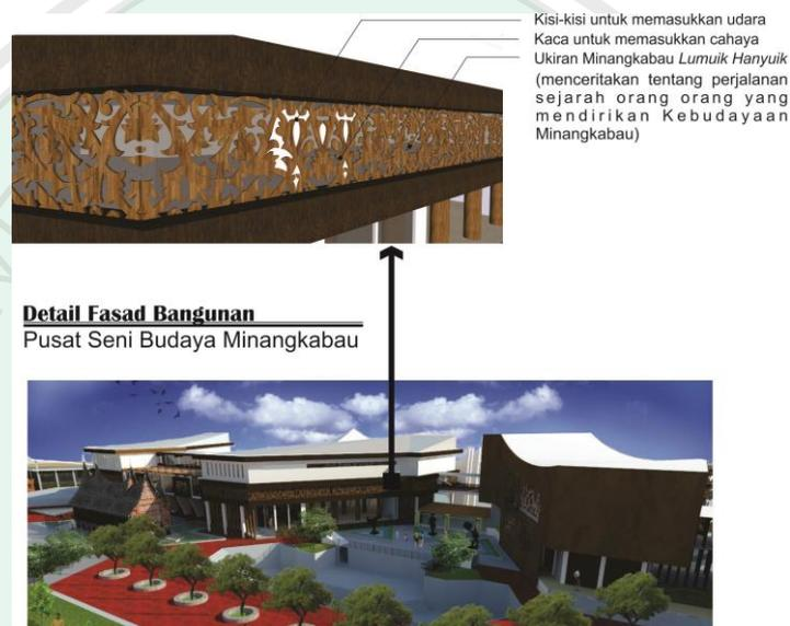
Gambar 6.27. Detail *shading device*
