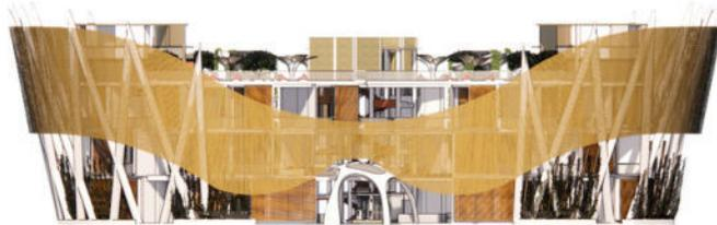
SECONDARY SKIN FACADE PADA BANGUNAN HOTEL INI MENGGUNAKAN MATERIAL ROTAN YANG DI ANYAM, MATERIAL INI MEMILIKI MASSA YANG RINGAN DAN DAYA TAHAN LAMA . FACADE ROTAN INI DI FRAMMING OLEH RANGKA BAJA RINGAN LALU DI TOPANG DENGAN PIPA BAJA.
