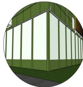
STRUKTUR BANGUNAN BETON KOLOM DI TAMPAKAN KE EKSTERIOR BANGUNAN HAL INI BERTUJUAN SEBAGAI ESTETIKA BANGUNAN DENGAN MENAMPAKAN STRUKTUR BETONNYA
