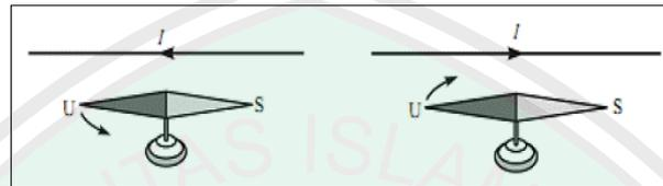
Gambar 2.7 Percobaan Oersted
