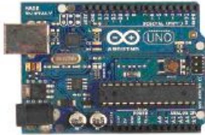
Gambar 2.2 Modul Arduino Uno
