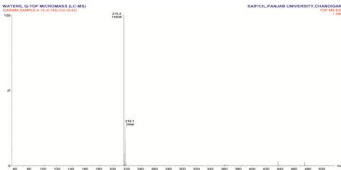
Fig. 7: Mass spectra for 4-chloro-N-benzylidene aniline obtained with grapes juice shows molecular ion peak and base peak
