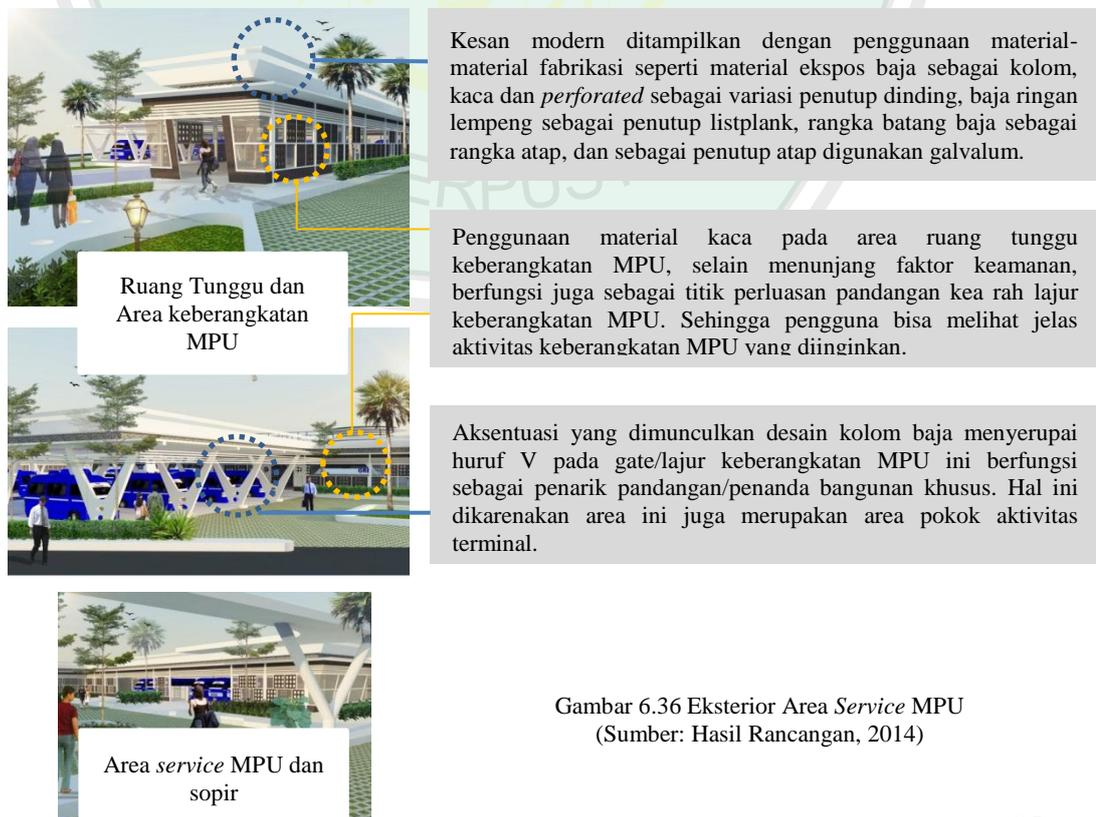
Gambar 6.36 Eksterior Area Service MPU
