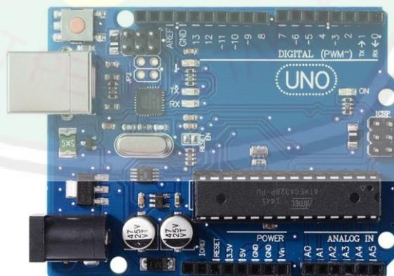
Gambar 2.4. Arduino Uno (Sumber: nanopowerbd.com)
