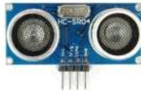
Gambar 2.1 Sensor Ultrasonik
