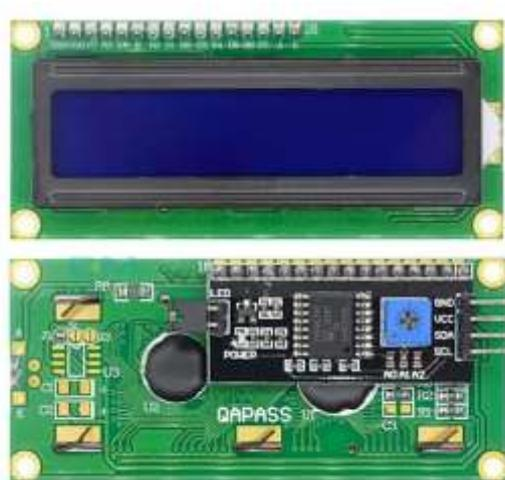
Gambar 2.19 *Liquid Crystal Display* 16 x 2 I2C (Odunlade, 2020)
