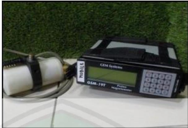
Gambar 2.17 Alat *Proton Precission Magnetometer* (Wibowo, 2017)
