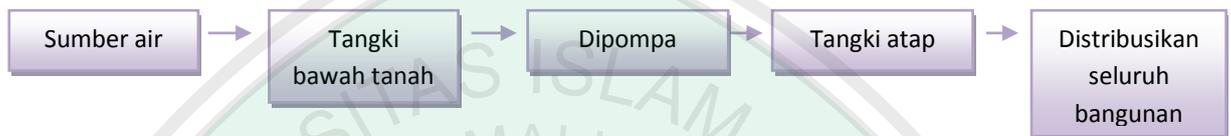
Gambar 4.22 Skema Alur Sistem Tangki Atap
