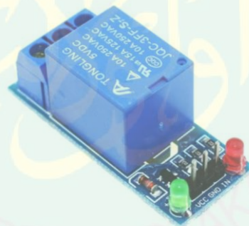
Gambar 2.8 Relay Modul (Safril, 2019)
