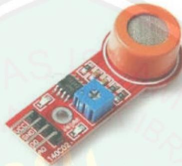
Gambar 2.1 Sensor Gas MQ-3
