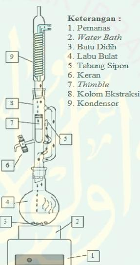
Gambar 2.4 Rangkaian Ekstraktor Soxhlet (Purwanto, dkk. 2014)
