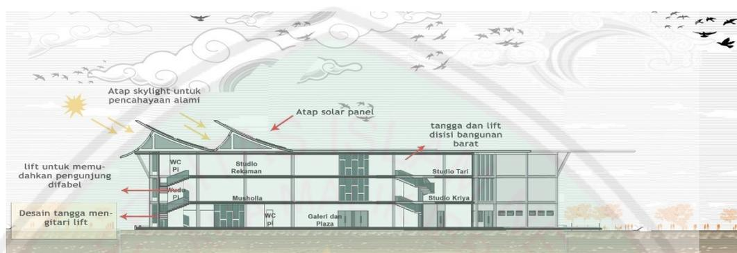
Gambar 6.39 Potongan A-A' Ged. Kesenian
