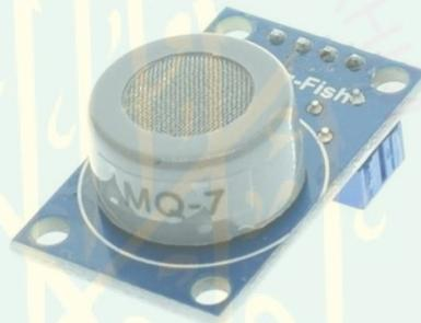
Gambar 2.1 Sensor Gas MQ-7
