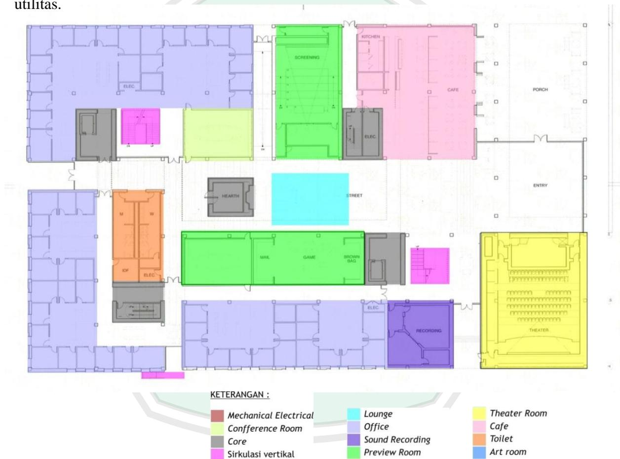
**Fig. 2.4.1.10** Detail Penzoningan Denah Lantai 1
