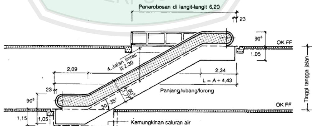
**Gambar 2.24 Detail Ukuran Eskalator**
