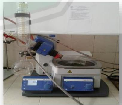
Gambar 6. Proses Rotary evaporator
