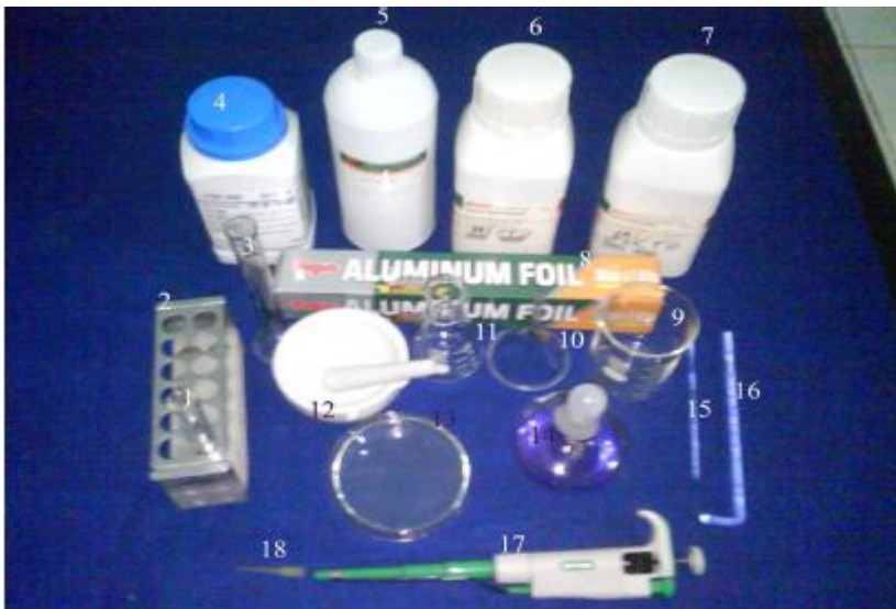
Gambar 4.8 1. Tabung Reaksi; 2. Rak Tabung Reaksi; 3. Gelas Ukur; 4. Medium SSA; 5. Alkohol 70%; 6. Pepton; 7. Beef extract; 8. Aluminium foil; 9. Beaker glass ; 10. Corong kaca; 11. Erlenmeyer; 12. Mortar; 13. Cawan petri; 14. Bunsen; 15. Jarum ose; 16. Spatel/spreader; 17. Micropipet; 18. Tip
